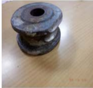
Damage sheave on accommodation ladder port side B
