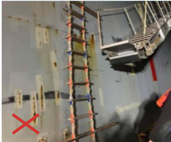
Distance of combination ladder from water line less than 5 metres
