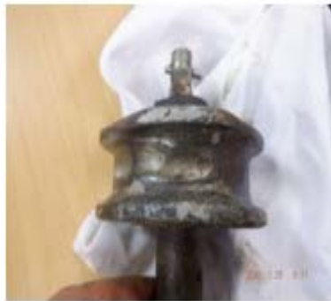
Damage sheave on accommodation ladder port side B
