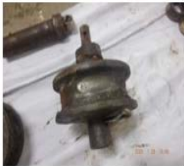
Dismantle the damage sheaves in portside accommodation ladder.
