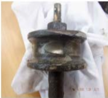
Damage sheave on accommodation ladder port side A
