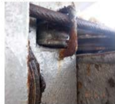
Damage sheave on accommodation ladder stbd side B( one piece)
